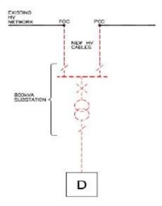
b) The Minimum Scheme is as for scenario a) above but the Customer requests an enhanced connection arrangement where the substation is looped into existing HV network
