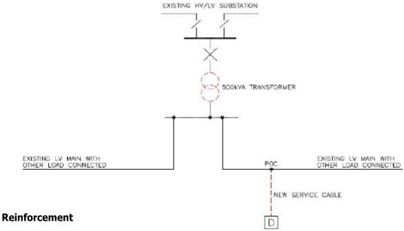
The RSN for the Reinforcement is the HV/LV transformer
